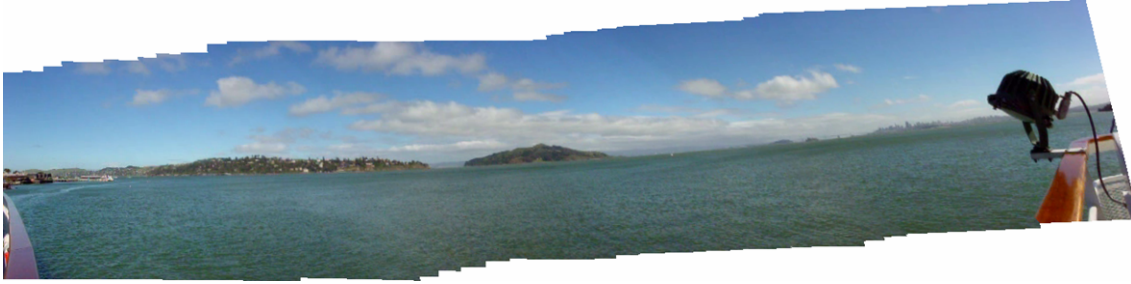
Fig. 4. Bending artifact using affine model.
