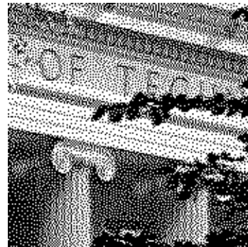
Figure 15. Improved error diffusion using a serpentine raster and a “noisy” weight filter.
