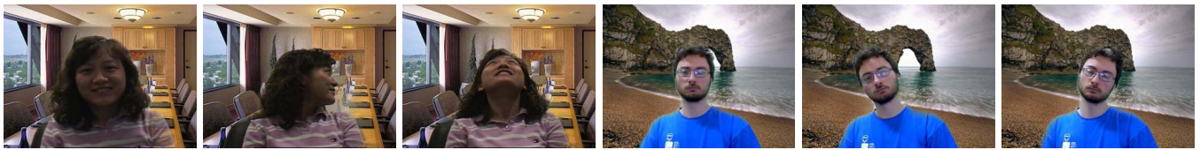
Fig. 7. Examples of background substitution using alpha matting.
