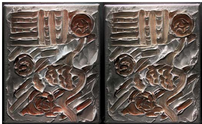
Figure 6. Canvas sample C1 before (left) and after (right) flattening of the impasto. Renderings from the PTM, showing the painting lit as though by raking light from the top: note the crushed impasto and impressed canvas weave
