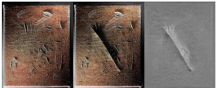
Figure 8. PTM renderings for canvas sample C3 before (left) and after (centre) scratching. The image to the right is the result of subtracting one of these renderings from the other
