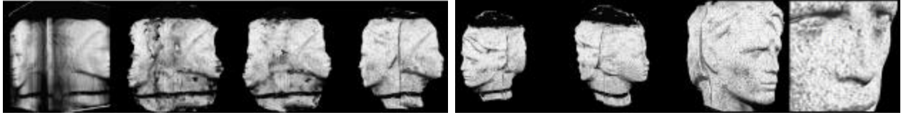
Figure 9. Reconstruction (left) and new view synthesis (right) of a two-headed object using the level set method. Images courtesy of Olivier Faugeras and Renaud Keriven.
