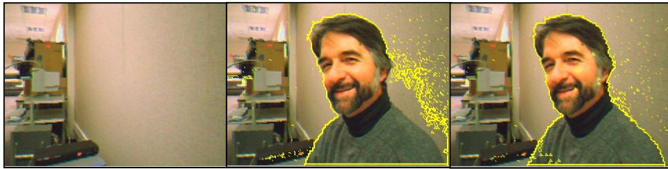
Figure 4. Left: background image; Center foreground contours; Right: foreground after shadow suppression.
