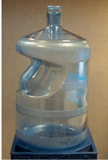
Fig.17. Bottle used as phantom for performance measurements
