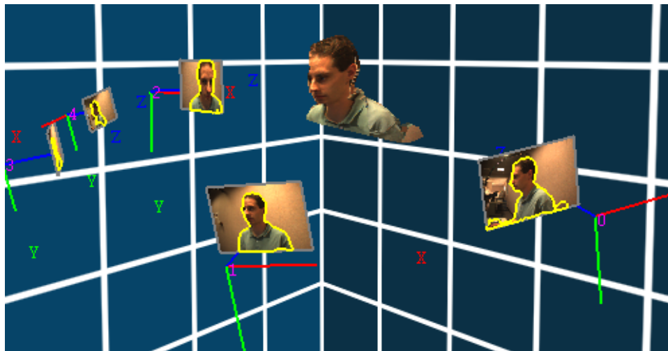
Figure 7. View of user in Coliseum space: Five cameras surround the rendered user. Each camera shows its coordinate system (in RGB), video frame, and foreground contour.
