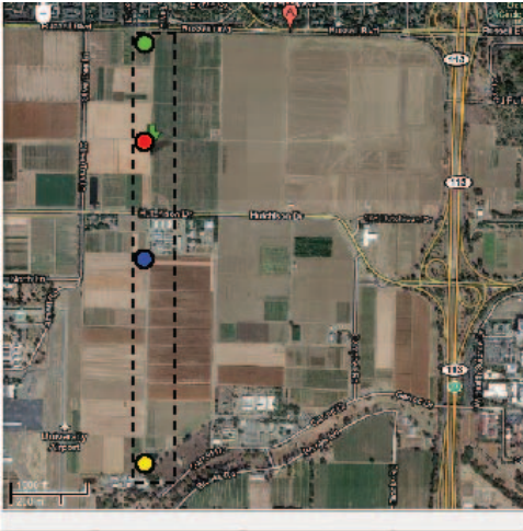
Fig. 7. Satellite view of the location where the experiment for the backhaul link testing is conducted. Node locations are shown using circles. The green node is kept fixed while the second node is moved to other locations to generate different link lengths.
