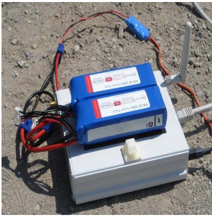
Fig. 2. Set up of a WCB node on the ground.
