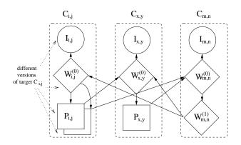
**Fig. 2.** Example of ILFS frame structure. I-, DSC and P-frames are denoted by circles, diamonds and squares, respectively. In this example, image  $C_{i,j}$  has four coded versions: I-frame  $I_{i,j}$ , DSC frame  $W_{i,j}^{(0)}$ , and two P-frames  $P_{i,j}(x, y)$  and  $P_{i,j}(m, n)$ .
