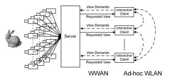
**Fig. 1.** System overview. A 2D array of closely spaced cameras capture spatially correlated images. Server encodes images into a frame structure. A client interactively requests images along her chosen trajectory from the server, while sharing displayed images with neighboring peers locally.
