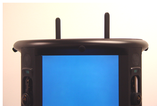
Fig. 6: A directional microphone is placed above each display in the surrogate head.
