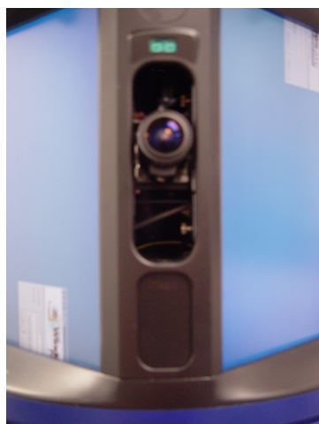
Fig. 5: A speaker port at the bottom of a vertical edge of the surrogate head. The speaker is covered with a black metallic speaker grille.
