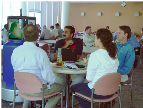
Fig. 8: A surrogate in use in a noisy cafeteria. Conversations in this environment would be difficult or impossible without multichannel audio.
