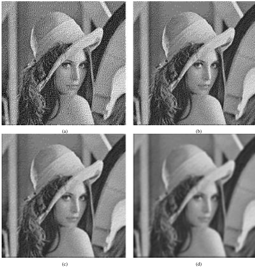
Fig. 2. Effect of the smoothing filter cutoff frequency on image smoothness. The Lena half-tone is filtered with three different filters from the family using the given parameters. The filter parameter x_2 is computed from x_1 using (2). (a) Original Lena half-tone. (b) x_1 = 1.40 \iff f_c = 0.46 f_N . (c) x_1 = 2.73 \iff f_c = 0.15 f_N . (d) x_1 = 3.40 \iff f_c = 0.065 f_N .
