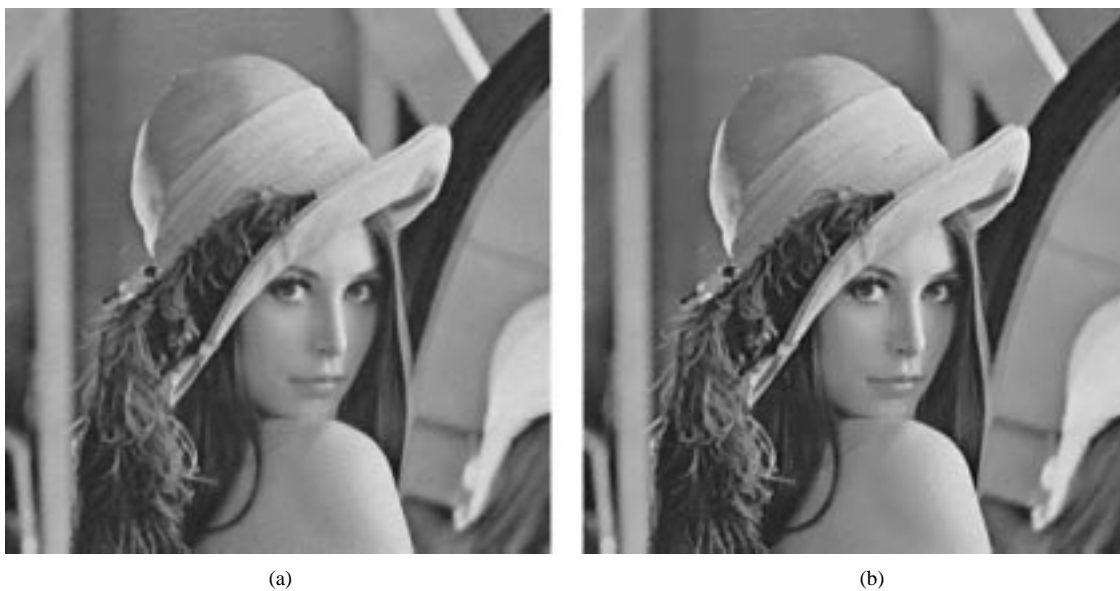
Fig. 8. Inverse halftoned Lena images. (a) Proposed algorithm, PSNR 31.34 dB. (b) Wavelet algorithm, PSNR 31.47 dB.
