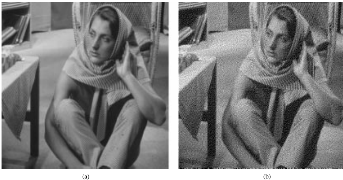
Fig. 11. Original Barbara image and its halftone. (a) Original image and (b) Floyd–Steinberg halftone.
