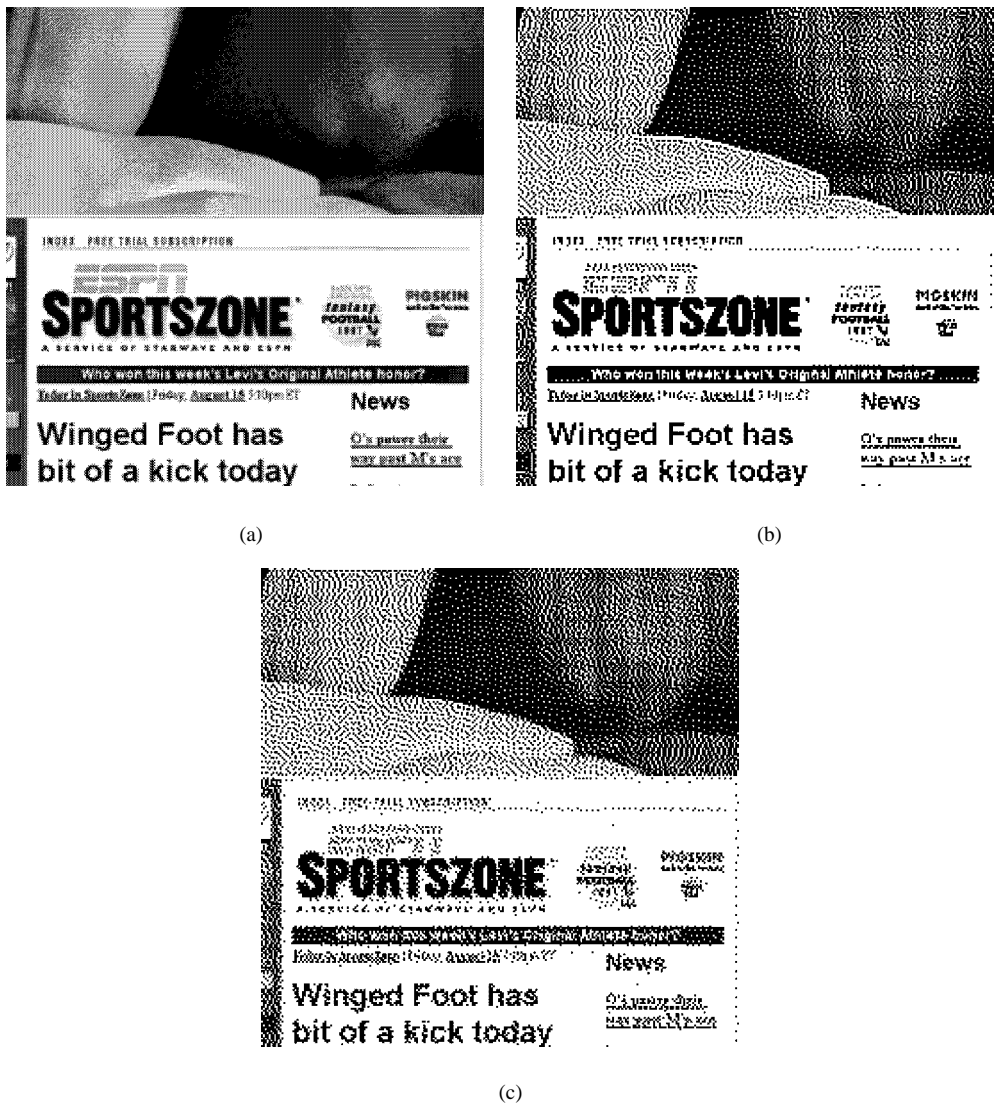
Fig. 11. Performance of the adaptive algorithm on a mixed document. (a) Original grayscale image, (b) result of Jarvis filter, and (c) result of using adaptive L .
