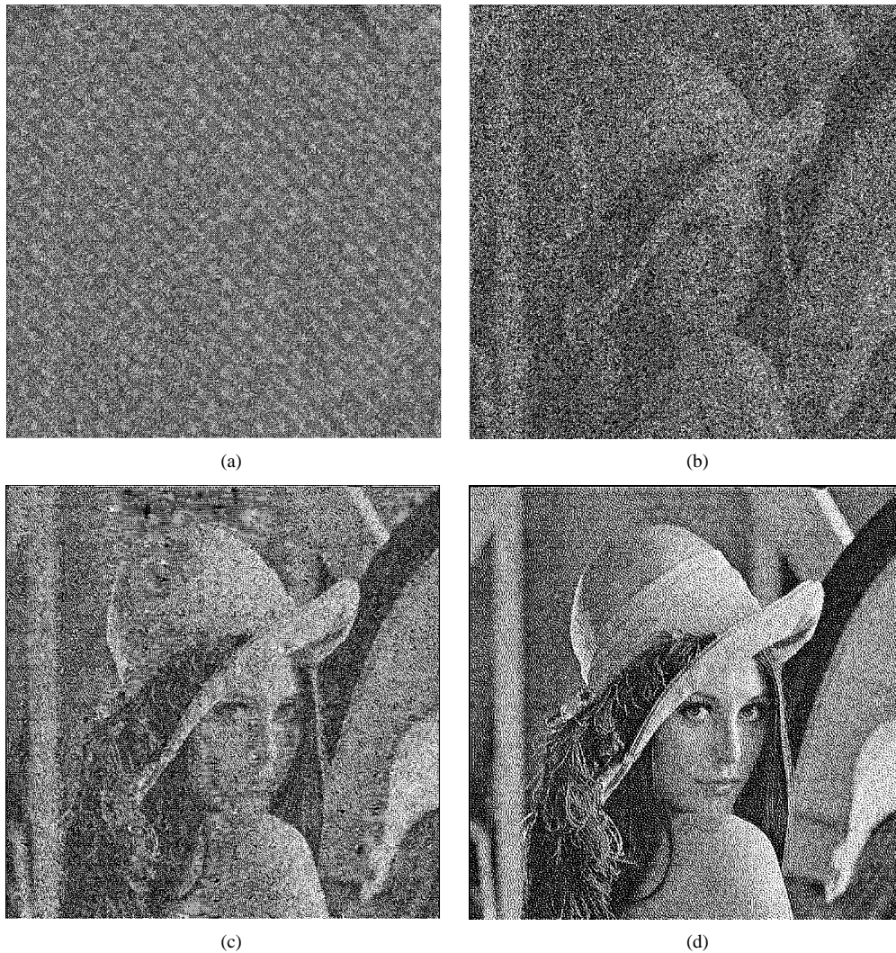
Fig. 15. Comparison of error images in various halftoning schemes. (a) Error image for adaptive DBF halftoning, (b) error image for nonadaptive DBF halftoning, (c) error image for fixed Floyd-Steinberg halftoning, and (d) error image for fixed Jarvis halftoning.
