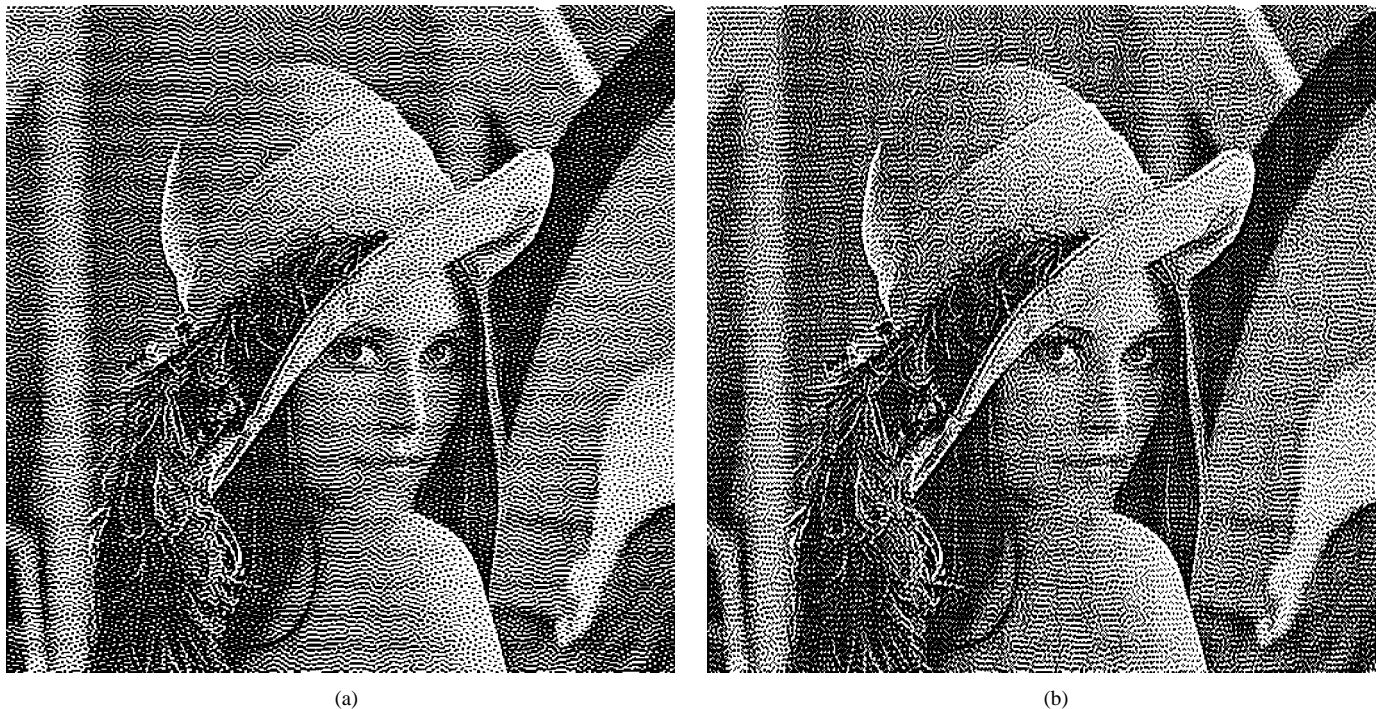
Fig. 18. Result of fixed and adaptive green noise halftoning on Lena image ( G = 0.5 ). (a) Floyd–Steinberg hysteresis filter and (b) adaptive hysteresis filter.
