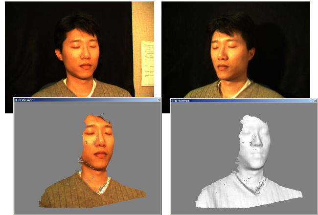
Figure 14. "Face2" image pair: reconstructed textured and untextured 3-D models.
