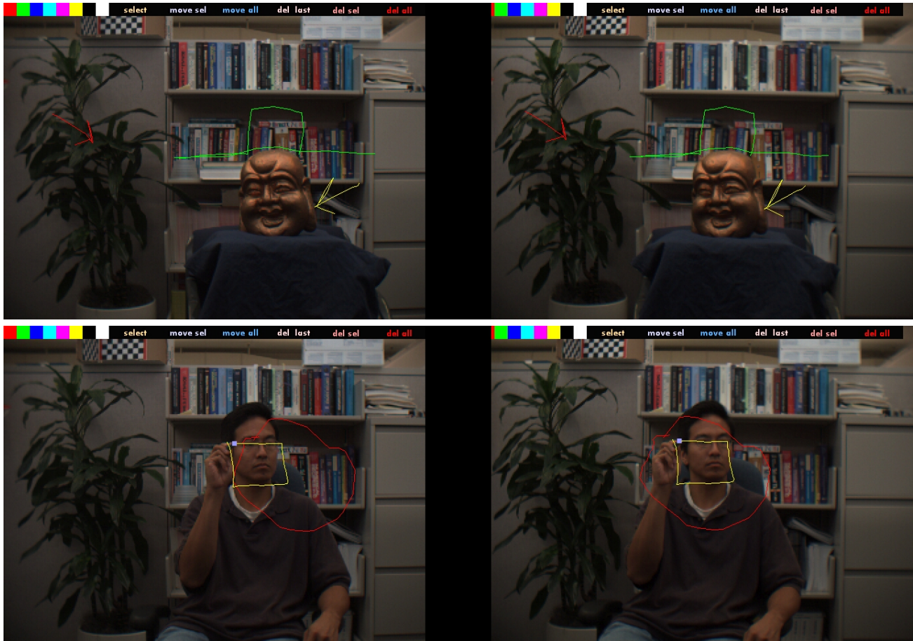
Figure 6. Virtual annotations in captured stereo pairs automatically appear at the correct relative depth in the scene.
