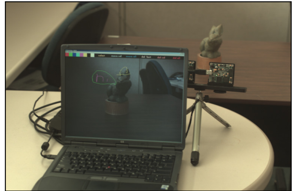
Figure 8. Example of prototype mixed-reality system with cameras oriented behind the display.
