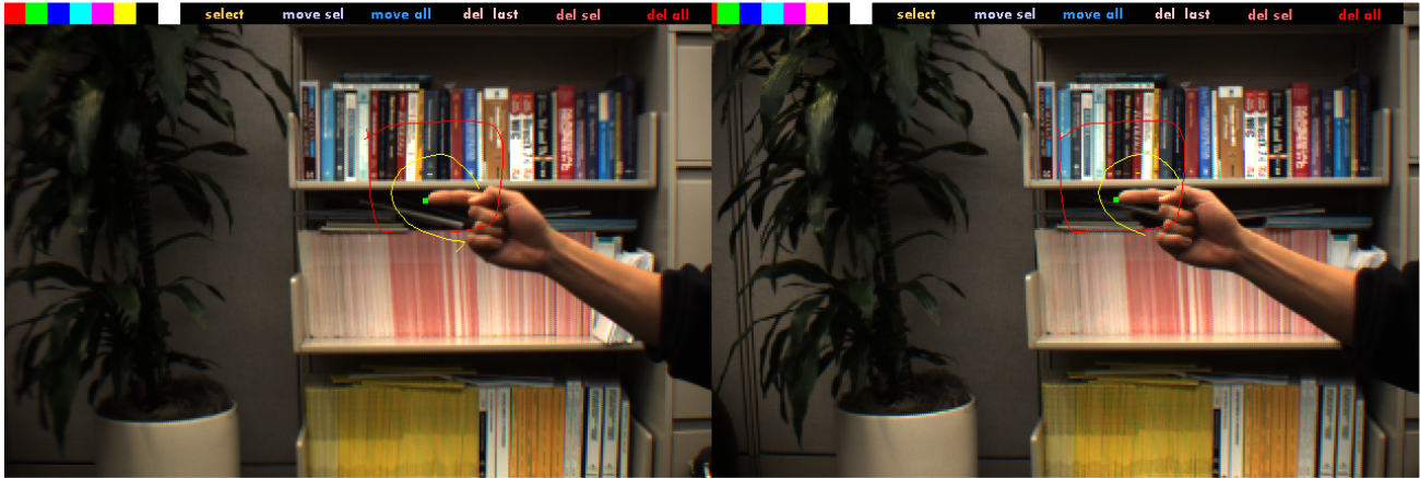
Figure 3. ArcSpace automatically preserves relative depth ordering between real and virtual objects in the scene.
