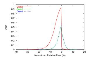
Figure 11: CPU allocation error, Credit, SMP case, 3 domains, NWC-mode, 66%:66%:66%.
