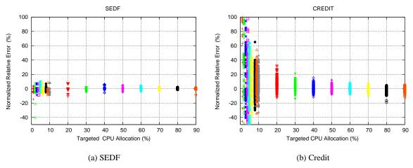
Figure 7: Benchmarking with ALERT: CPU allocation error under SEDF versus Credit schedulers in Xen.
