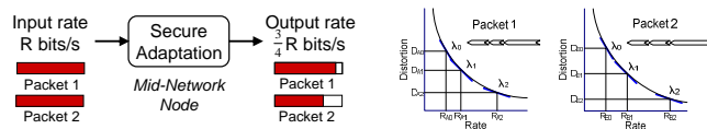
Fig. 2. R-D optimized secure adaptation across two packets is achieved by appropriately truncating each packet so that they operate at the same slope \lambda on their R-D curves.
