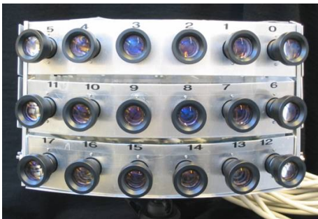
Figure 1: A mosaic camera is one type of new video application enabled by current imaging and computing trends.
