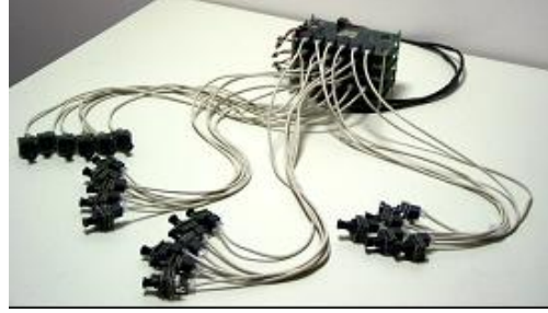
Figure 4: Our capture hardware currently supports 22 Bayer-format VGA cameras at 30 Hz, without compression.
