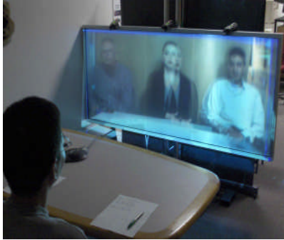
Figure 9. Multi view zone projection display.
