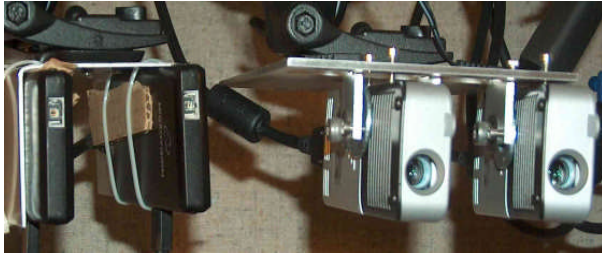
Figure 7. A pair of Microvision (left) and 3M (right) pico projectors assembled in a binocular stereo mode.
