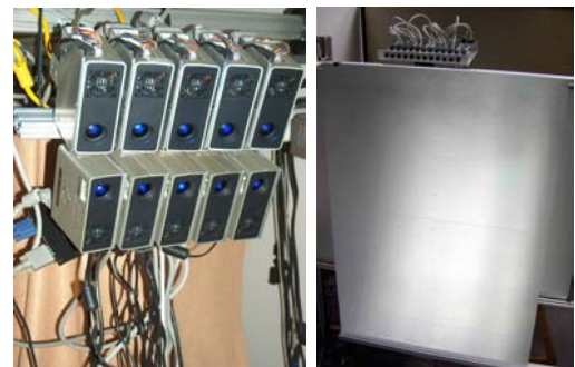
Fig. 2. Autostereo display: (left) above-viewer pocket projectors; (right) diffusing retroreflection screen
