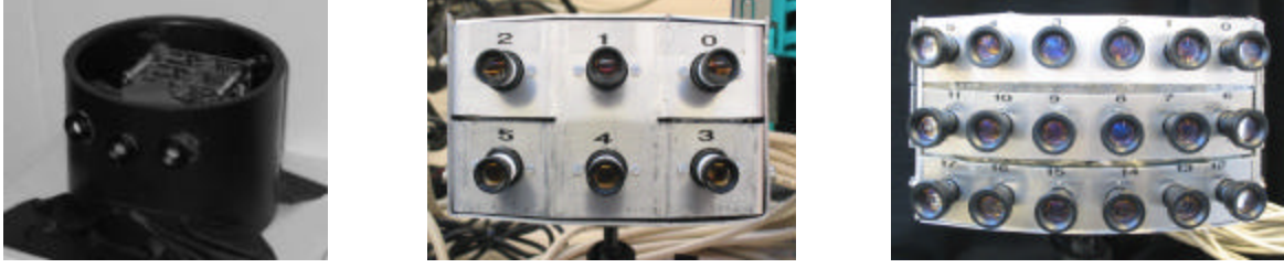
Figure 5: Panoramic camera configurations: (a) 1 MPixel, (b) 2 MP, (c) 6MP
