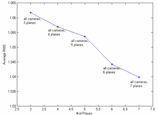
Figure 4: Reduction in RMS error with increasing number of homology constraints.
