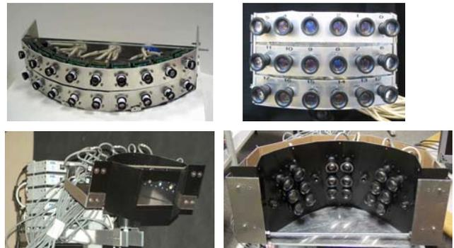
Figure 1: Multi-imager camera arrays.
