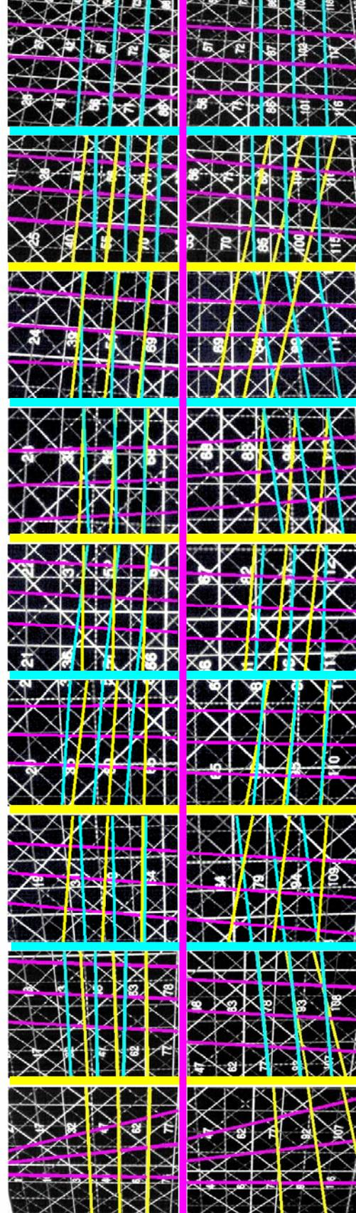
Figure 3: Corresponding epipolar lines for 2x9 multi-imager configuration: yellow-cyan alternating horizontally, magenta vertically
