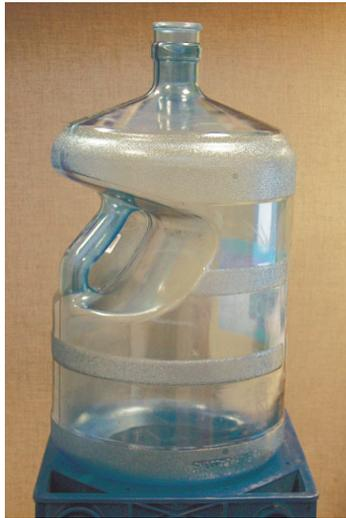
Fig. 17. Bottle used as phantom for performance measurements.
