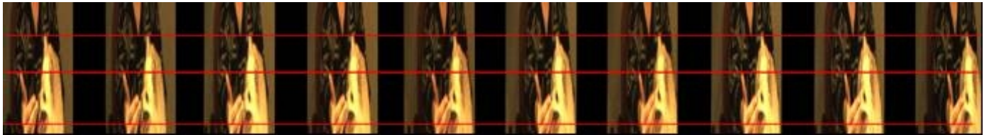
Figure 5. Rectification Result – epipolar lines across 10 imagers through the three selected features
