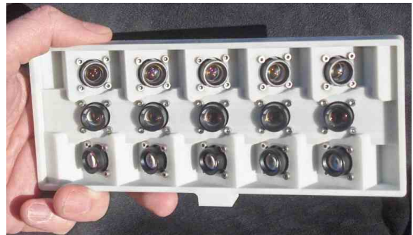
Figure 1. Simultaneous panoramic+multiview camera
