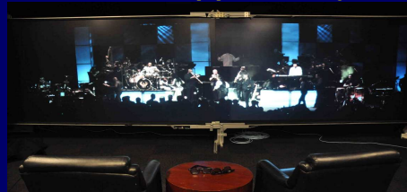
Prototype 22'x6' double-wide HD (3840x1080 @ 60 fps) 3D display using eight tiled+superimposed projectors.
