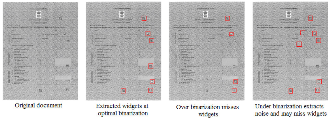
Fig. 3. Proposed adaptive binarization for robust widget extraction irrespective of background textures or print/scan variations.
