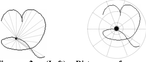
Figure 2: (Left) Distances from a point (highlighted) to rest of the points. (Right) Shape Context feature with 4 r -bins and 10 \theta -bins at the point considered.
