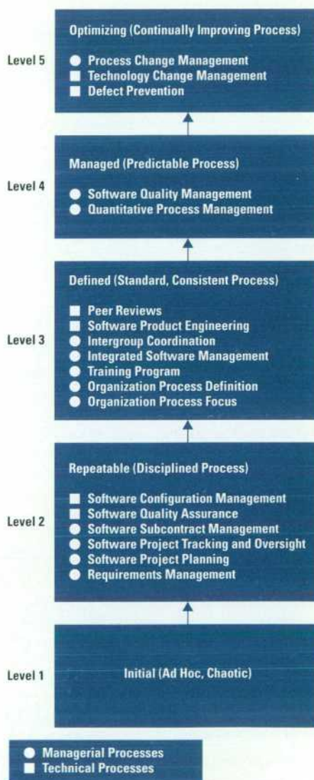
Fig. 1. The five levels of the Capability Maturity Model (CMM). The items listed at each level are called key process areas. These areas determine an organization's software development maturity.
