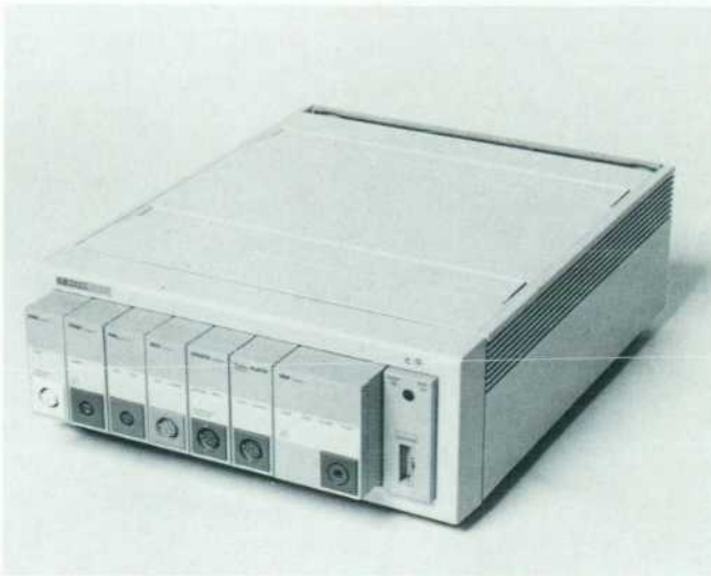
Fig. 4. Assembled computer module with integral parameter module rack.
