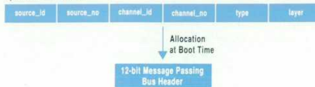
Fig. 6. Every message has a composite symbolic identification, which is evaluated at boot time, when message headers are allocated.
