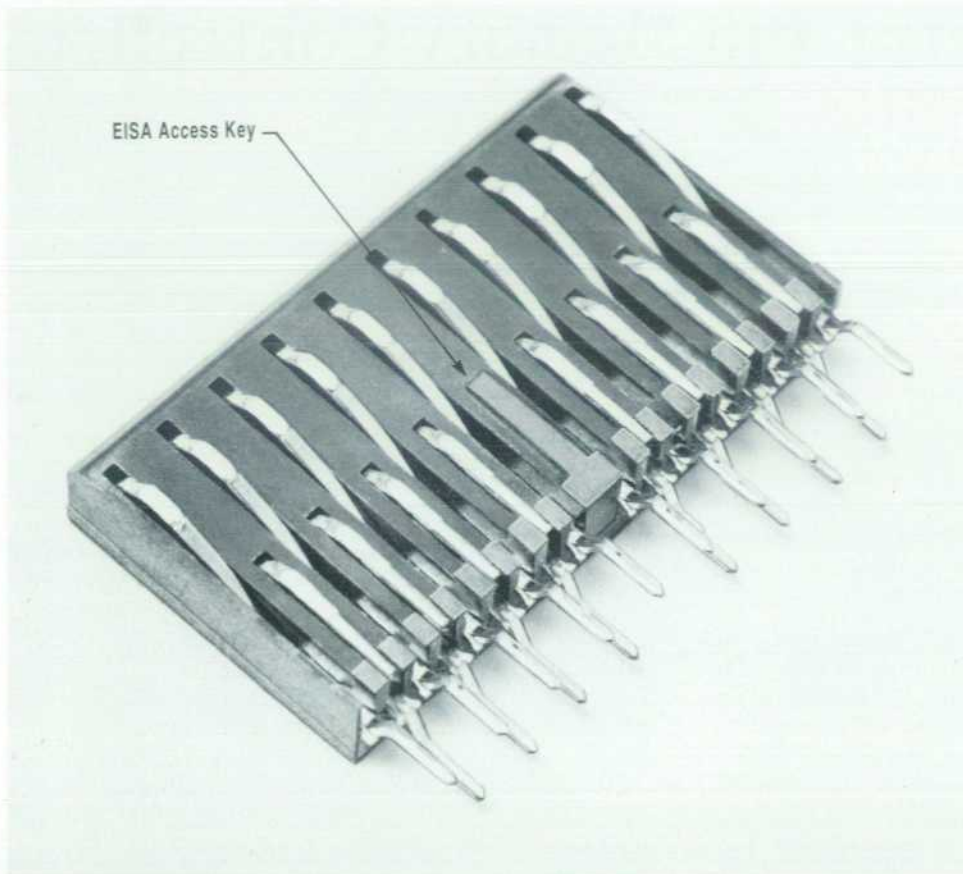
Fig. 5.* Inside view of one half of an EISA connector. The EISA access key prevents ISA boards from being inserted to the depth of the EISA contacts.
