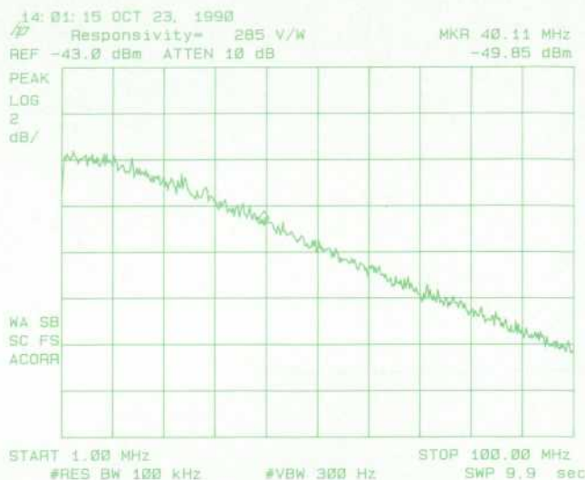
Fig. 12. Linewidth measurement of a single-frequency distributed feedback laser.
