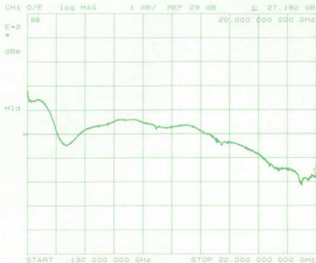
Fig. 9. Lightwave receiver frequency response.
