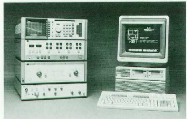
Fig. 5. HP 83420A lightwave test set with the HP 8510B microwave network analyzer.
