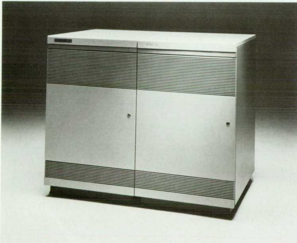
Fig. 2. The HP 3000 Series 930 Computer is the first HP Precision Architecture computer for commercial applications. Its operating system is HP's proprietary MPE XL.
