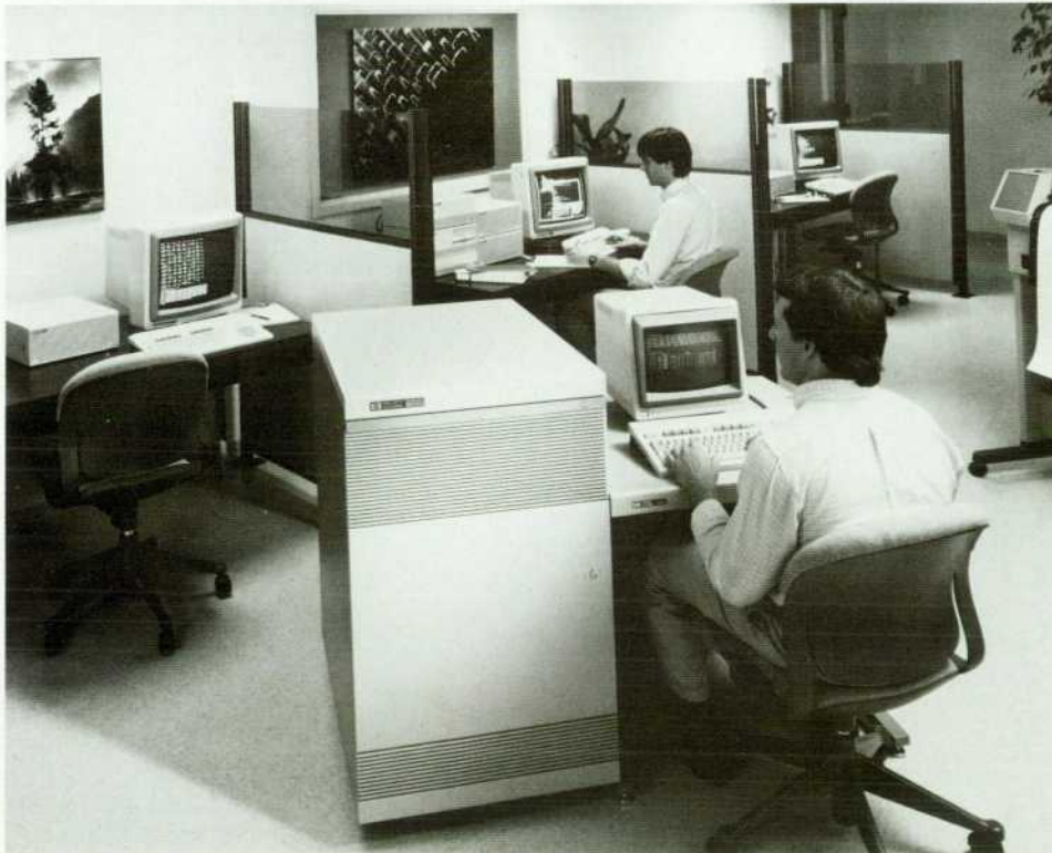
Fig. 1. The HP 9000 Model 840 Computer is the first HP Precision Architecture computer for technical and real-time applications. Its operating system is HP-UX, HP's version of AT&T's UNIX System V operating system.
