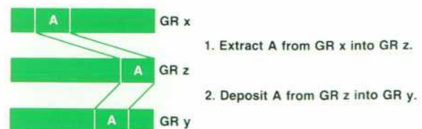
Fig. 7. Movement of an arbitrary field using extract and deposit instructions.
