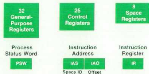
Fig. 2. HP Precision Architecture processing resources are organized around three register arrays and a few specialized registers.
