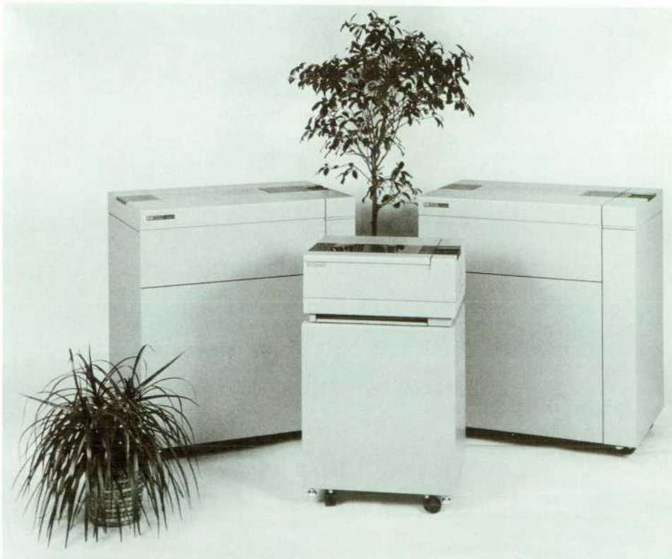
Fig. 1. The HP 2563A (foreground), HP 2565A, and HP 2566A Line Printers are dot matrix impact printers that operate at speeds of 300, 600, and 900 lines per minute, respectively. High reliability and print quality and low cost of ownership were primary design objectives.
