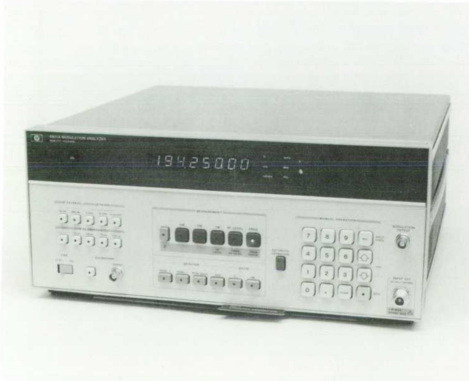
Fig. 1. Model 8901A Modulation Analyzer measures a signal's frequency, drift, power, AM, FM, and residual noise. It also recovers the modulating signal. Its carrier frequency range is 150 kHz to 1300 MHz and its modulation depth or deviation measurements are generally accurate within one percent of reading.
