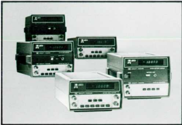
Fig. 2. Model 3470 Measurement System consists of display section and various signal-conditioning sections (two at time of writing) plus battery and BCD output sections which fit together in combinations to suit differing users' needs.
