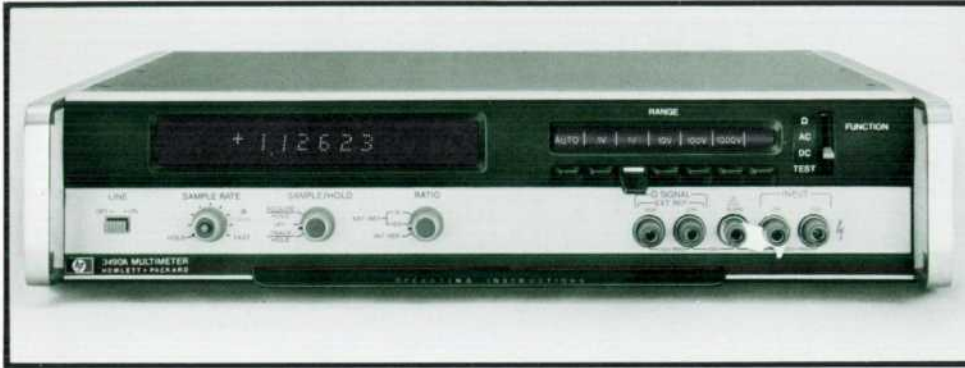
Fig. 1. Model 3490A Digital Multimeter measures dc volts, ac volts and resistance with 10 ppm resolution. Model shown here has Ratio and Sample-and-Hold options installed. Easy-to-decipher range and function control brings into view only those ranges needed for function selected. Depressing appropriate tab selects range desired. Slide-out instruction card includes operator instructions for using Multimeter to test itself.
