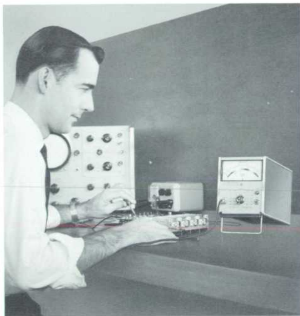
Fig. 1. Hewlett-Packard Model 3400A RMS Voltmeter indicates root-mean-square value of complex waveforms having frequency components within 10 cps to 10 Mc passband. Large crest factor of 10 to 1 enables accurate rms voltage measurements on nearly all waveforms, including impulse noise and narrow pulse trains (see text).
