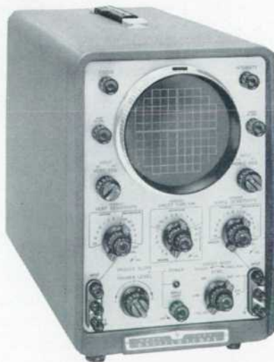
Fig. 1. New hp -Model 130A DC-300 KC Oscilloscope has been designed with special emphasis on its suitability for measuring voltage, time, and phase shift. Special features include high sensitivity and stability, triggered type sweep with automatic triggering, identical vertical and horizontal amplifiers.
