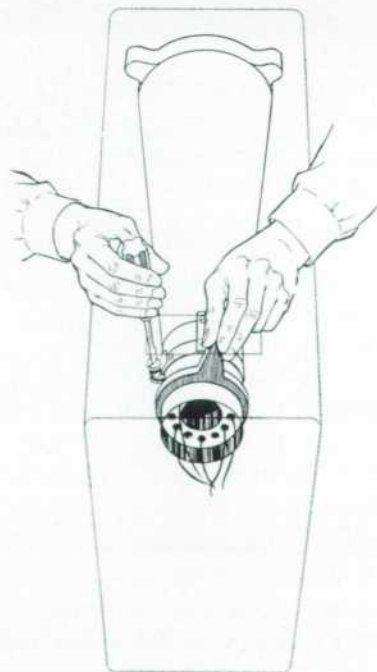
Fig. 14. Crt socket is provided with positioning lever to facilitate angular positioning of tube.
