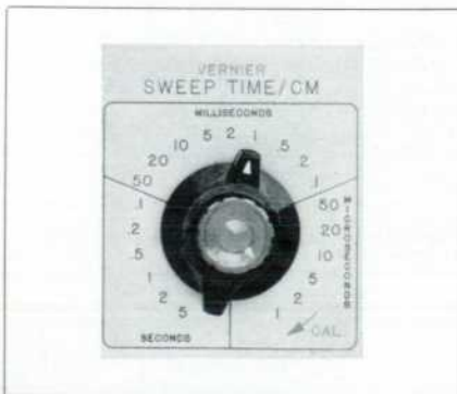
Fig. 6. Sweep Time control is direct-reading. Concentric knob is 3:1 vernier for selecting intermediate sweep times.
