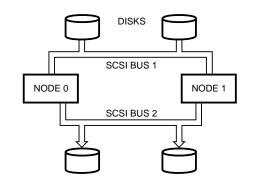
**Figure 5** Typical ASE Configuration
