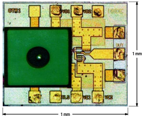
The solder bump interconnection is completed by solder reflow at 240°C in a nitrogen atmosphere using a clamshell type oven. The oven provides very stable and repeatable annealing conditions from run to run. The reflow time is 45 seconds, which includes 15 seconds of ramp time and 30 seconds of dwell time.
