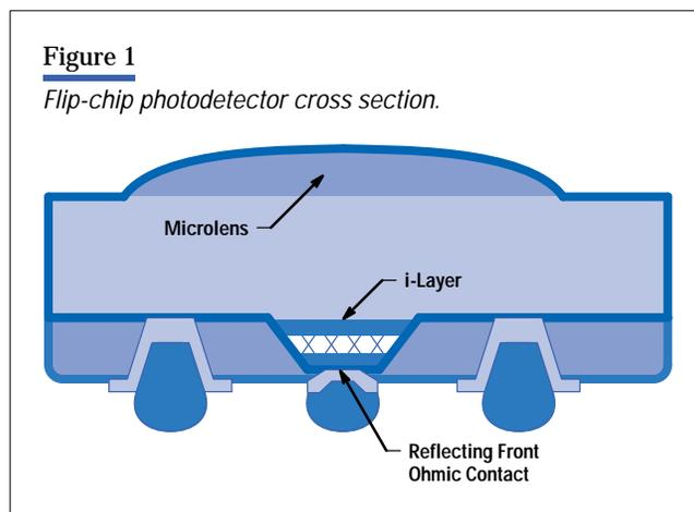
By a combination of the flip-chip packaging concept and device geometry optimization we can meet the required system goal. The flip-chip die attachment technique provides the following advantages to the design and performance of a high-speed photodetector:
