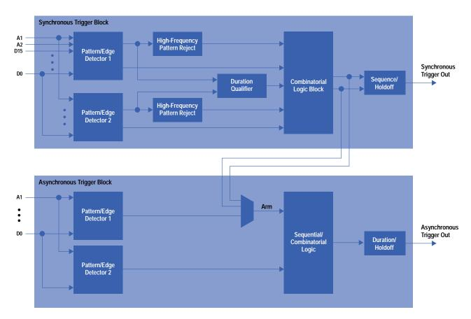
Fig. 5. HP 54645D trigger system block diagram.
