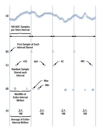
Fig. 3. Various decimation techniques shown at 100:1 oversampling. (a) ADC samples. (b) Simple decimation. (c) Intra-acquisition dither. (d) Peak detection. (e) Smoothing.
