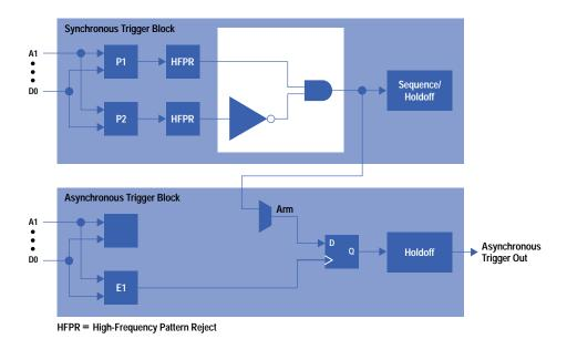
Fig. 7. Cross-domain trigger configuration.
