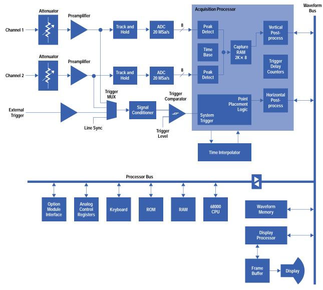
Fig. 1. Original HP 54600 Series oscilloscope block diagram.
