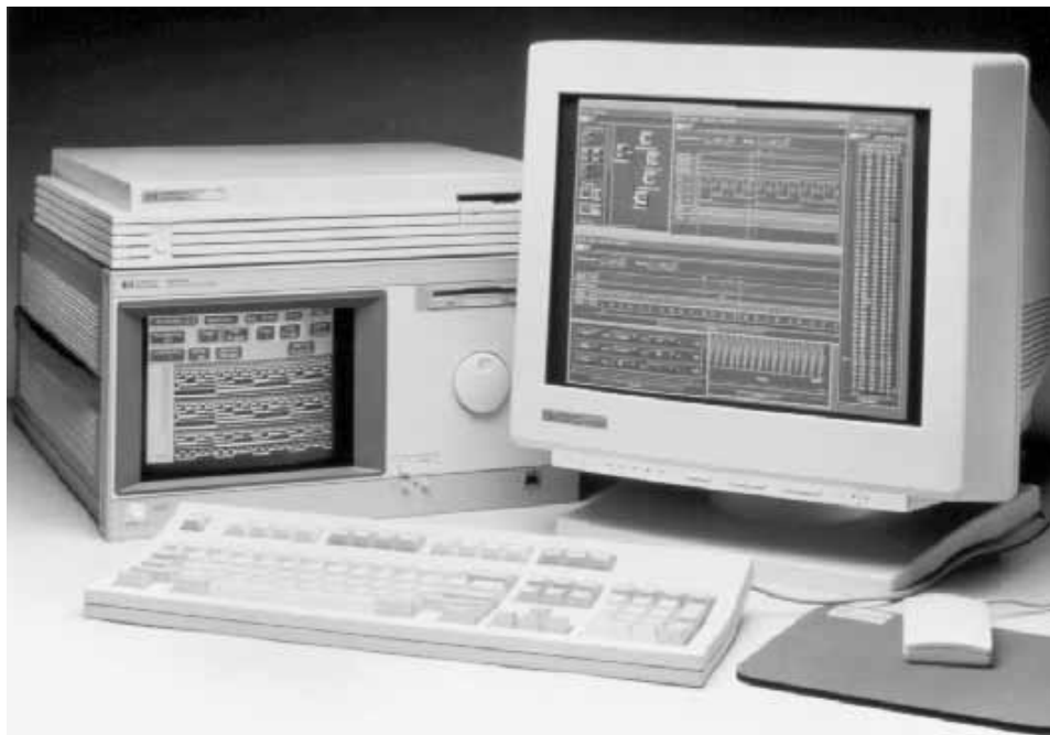
Fig. 11. HP 16505A prototype analyzer.
