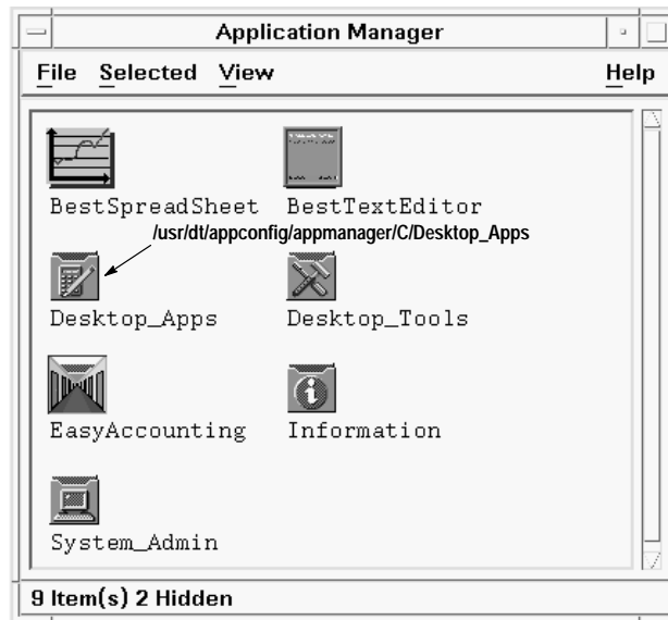
Fig. 4. The Desktop_Apps application group is a built-in group provided by the desktop.
