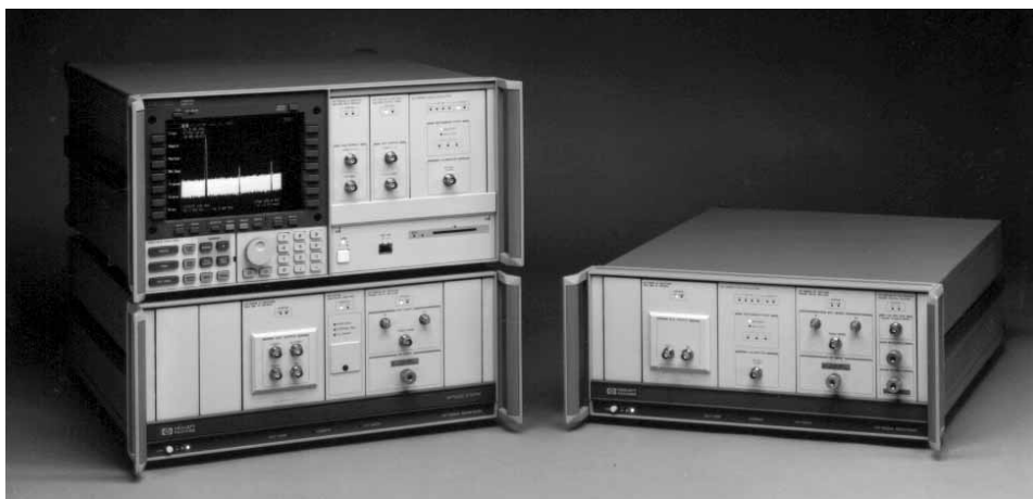
Fig. 1. (left) HP 71910A receiver. (right) HP 71910A Option 011 (a display module like the one at right may be added).
