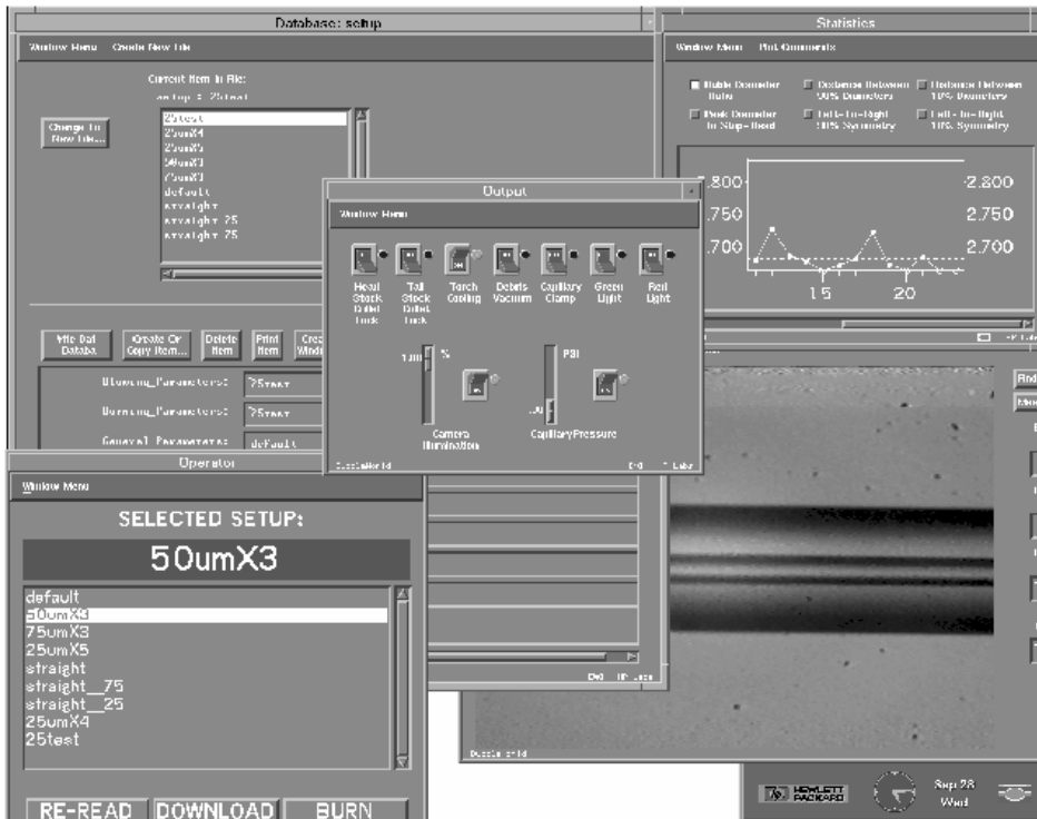
Fig. 7. A custom graphical user interface (GUI) was designed to allow the user to develop, execute, and monitor the manufacturing process easily. There are windows for setting up parameters, collecting statistics, and displaying live video of the forming bubble.
