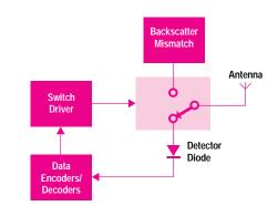
Fig. 1. Typical transponder block diagram for backscatter RF/ID technology.
