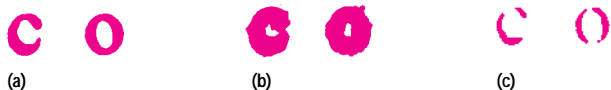
Fig. 3. The results of different threshold settings. (a) Normal setting. (b) Threshold set too low. (c) Threshold set too high.
