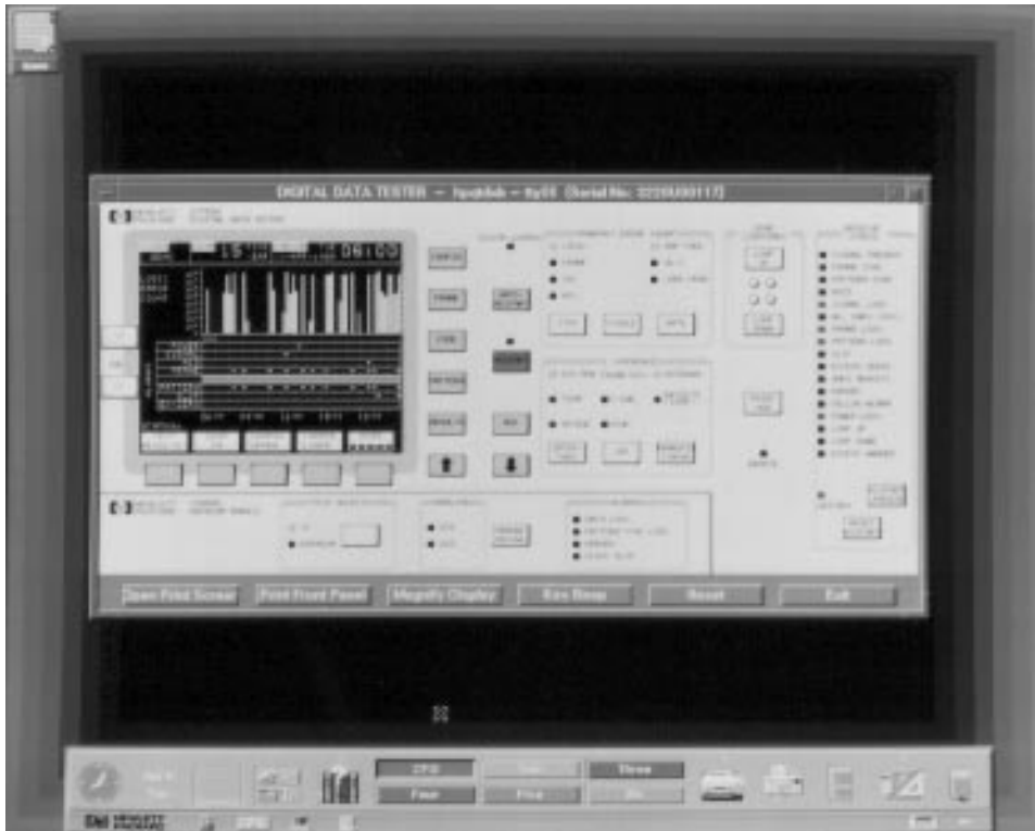
Fig. 6. A workstation screen displaying a picture of an instrument drawn by the virtual remote application. All of the data used to draw this image is stored in the instrument and is sent to the virtual remote application when requested. This allows virtual remote to be used with many different instruments without having any special knowledge about how they look or operate.
