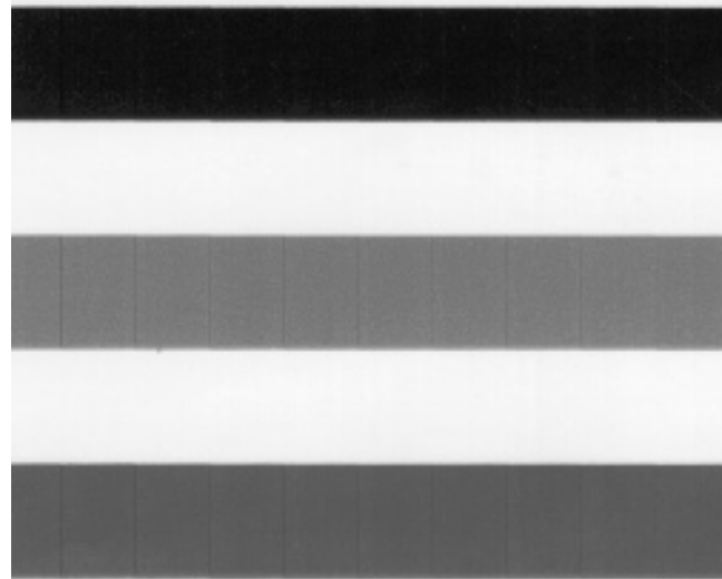
Fig. 1. Drop placement errors caused by swath advance.
