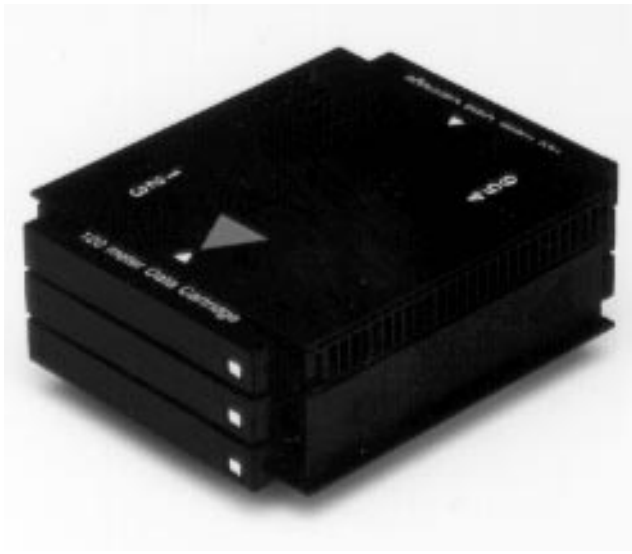
Fig. 2. The six-cartridge magazine is designed to be handled like one large tape cartridge.
