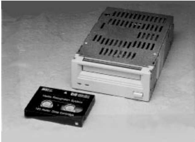
Fig. 2. The HP C1533A DDS-2 tape drive has a native-mode data transfer rate of 510 kbytes/s, 40% faster than other designs. It records on high-capacity 4-Gbyte DDS-2 cartridges or on earlier DDS media.
